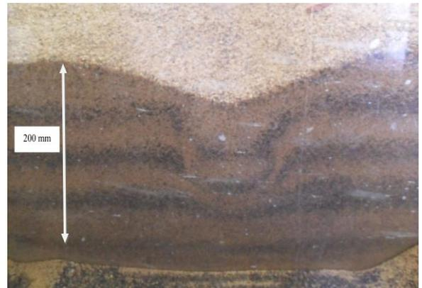
Figure 9: Failure pattern of soil body underneath to the square flat footing
