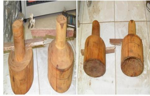
(i) Circular flat and its counterpart shell (conical) foundations
