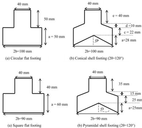
Figure 1: Sketch model of foundations
