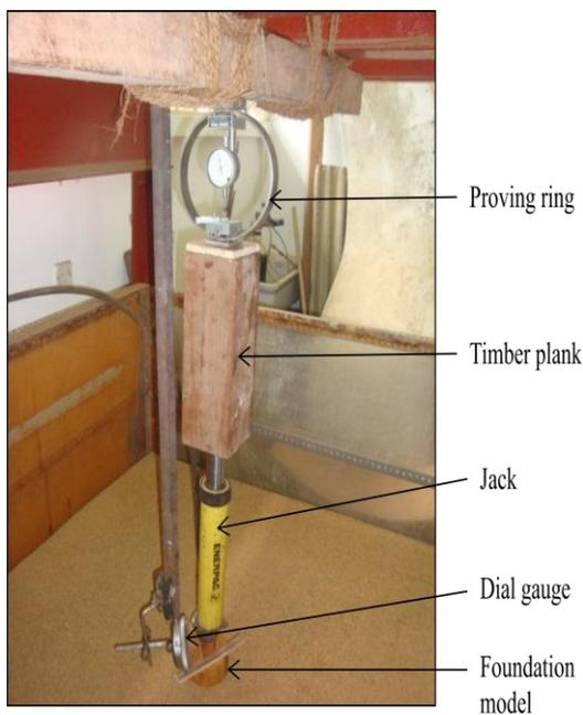
Figure 4: Load and settlement measurement set up
