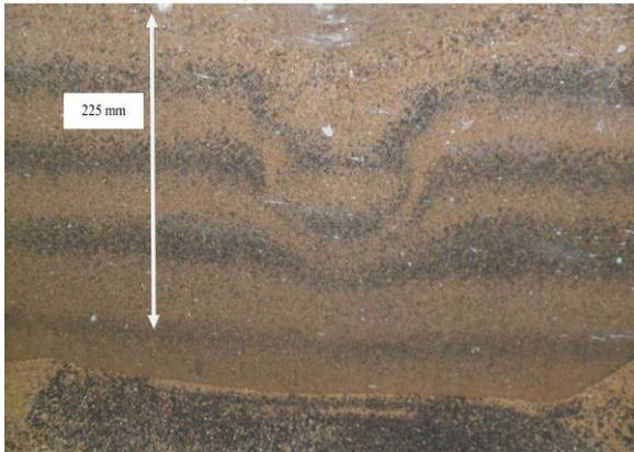
Figure 7: Failure pattern of soil body underneath to the circular flat foundation
