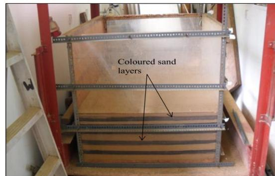
Figure 3: The perspex testing box with coloured and non - coloured sand layers
