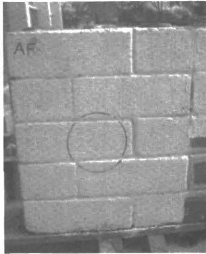
Figure 1: Acrylic filler applied on a test panel made out of interlocking blocks
