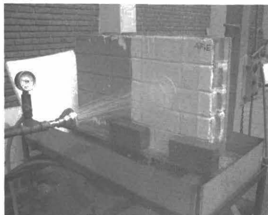
Figure 9: Erosion test on a wall panel made out of CSEB
