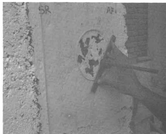
Figure 8: Measuring the pit depth inserting a rod (10 mm diameter flat ended)
