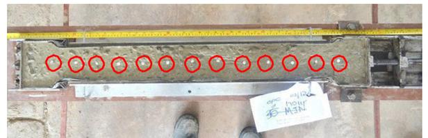
Figure 2: Fresh concrete sample with markers
