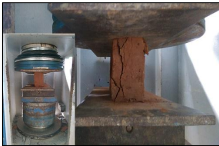
Figure 3: Testing of Bricks using Concrete Crushing Machine
