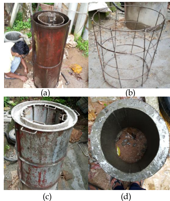
Figure 2.2: Casting procedure of cylindrical culverts; (a) Assembling of the mould, (b) Steel reinforcement cage, (c) Concreting, (d) Curing
