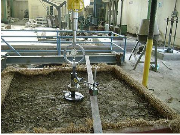
Figure 6: Loading arrangement for Plate load test
