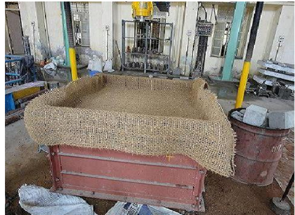
Figure 5: Coir geotextile at mid-depth of subbase
