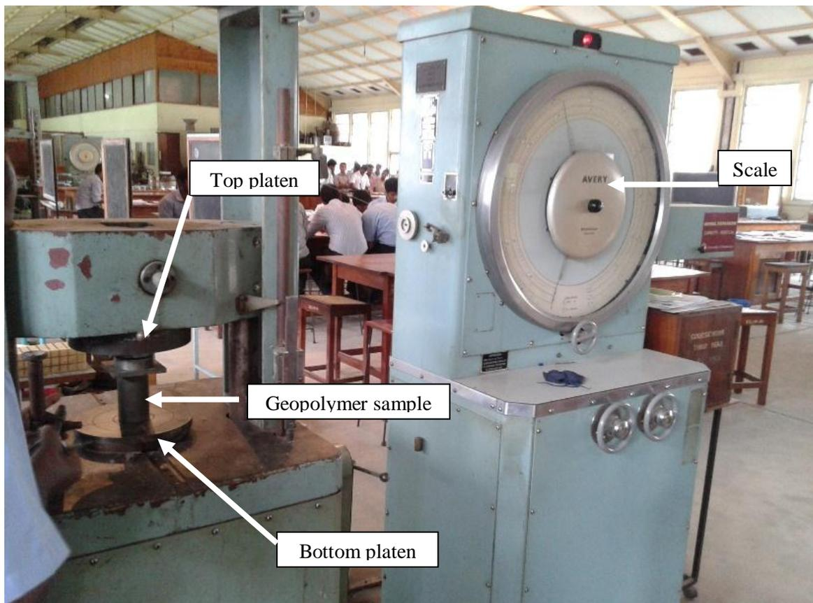
**Figure 3:** schematic view of UCS testing machine
