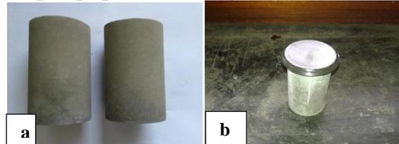
**Figure 2:** (a) Oven cured geopolymer samples, (b) sulphur capped sample
