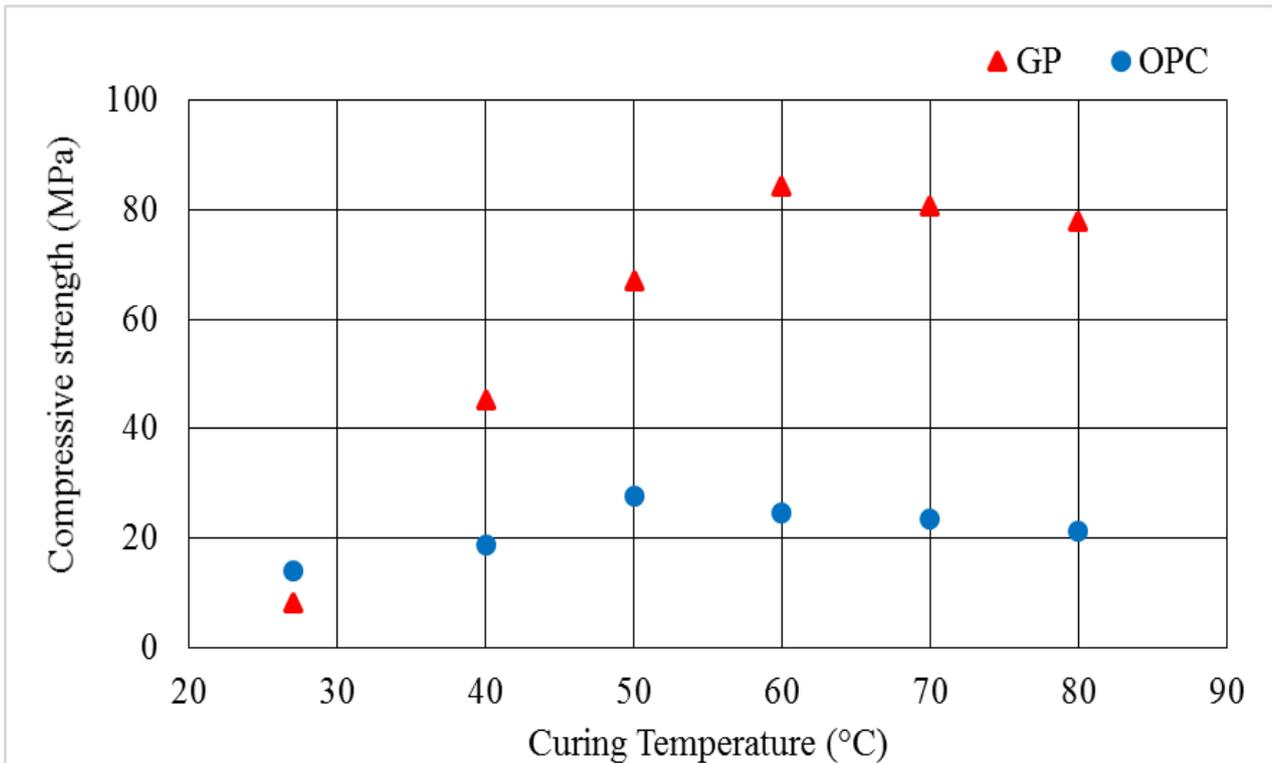
**Figure 5:** Variation of UCS with curing temperature for geopolymer and OPC
