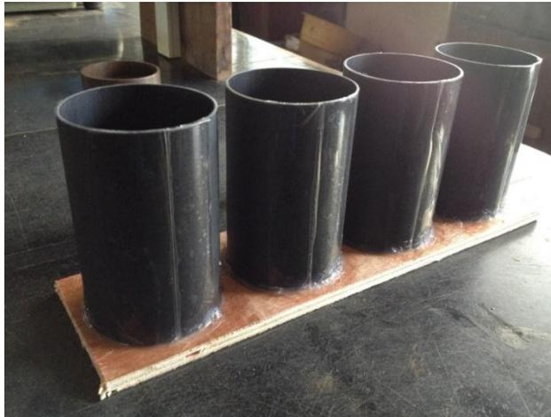
**Figure 1:** PVC moulds used to caste cement samples
