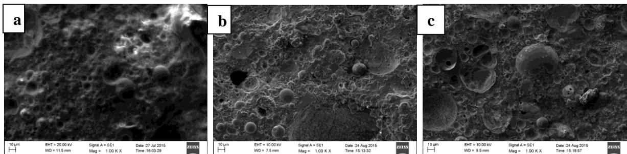
**Figure 9:** SEM images of geopolymer samples cured at 60 °C for (a) 2 days, (b) 7 days, (c) 14 days
