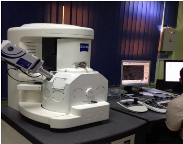
**Figure 4:** SEM testing machine used
