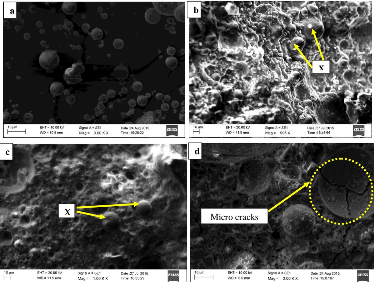
**Figure 8:** SEM images of (a) fly ash particles (a), geopolymer cured at (b) RT, (c) 60 °C and (d) 80 °C
