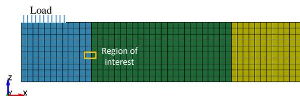
Figure 7: Reduced mesh for evaluation of contact interface.
