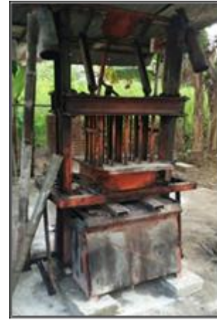
Figure 2: Local block manufacturing machine
