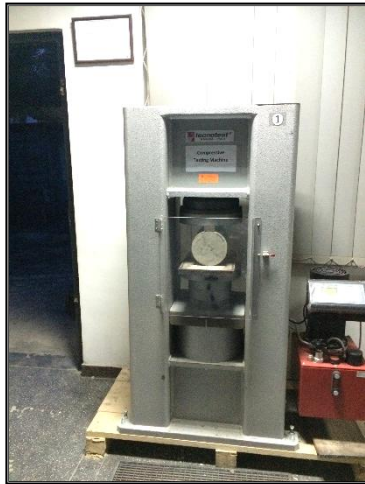
Figure 2 Split tensile test
