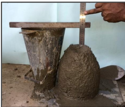
Figure 3 Measuring the Slump
