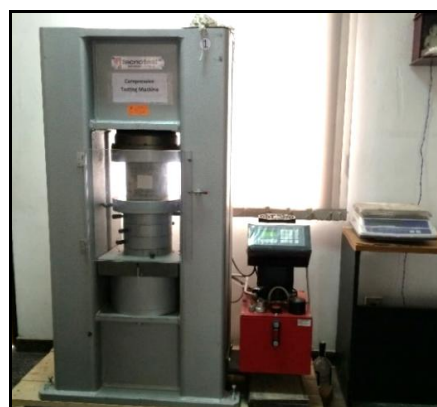
Figure 1: Compressive strength testing
