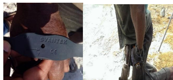
Figure 2: Measuring procedure of hand arm vibration exposures (a) Sensor was placed on the hand (b) Measuring the exposure levels
