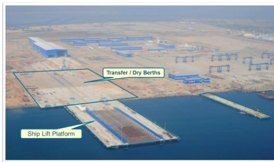
Figure 4: Layout of Shiplift facility
