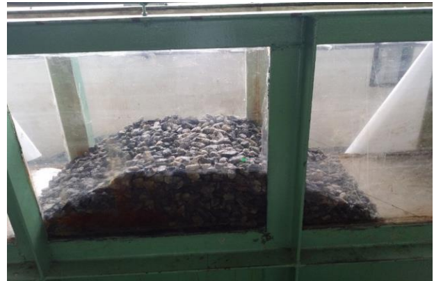
Figure 4: Breakwater model for 40 cm crest width using 26 mm armor units
