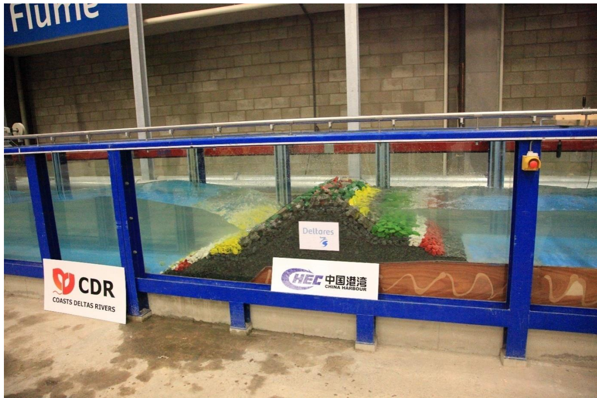
Figure 8: Set up of 2D physical model test to determine the characteristics of the offshore breakwater
