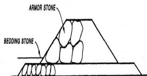
Figure 1: Typical cross section of a reef breakwater
