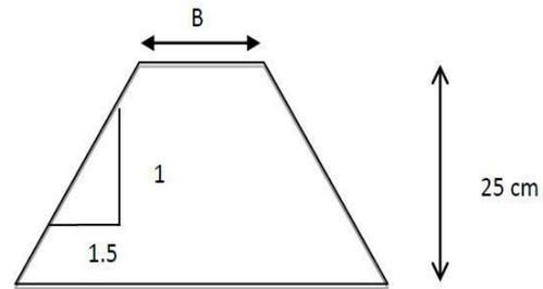
Figure 3: Cross section of a model breakwater
