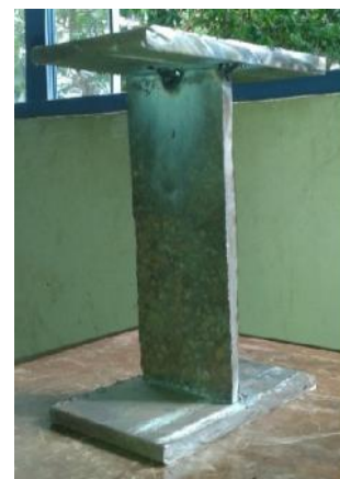
Figure 2: Prepared specimen for the compression test
