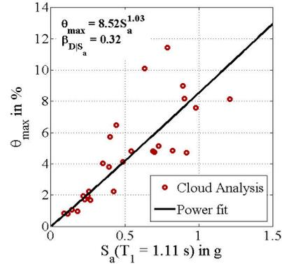
Figure 3: The power-law relationship between the interstory drift and spectral acceleration (adopted from Rajeev and Tesfamariam [21])
