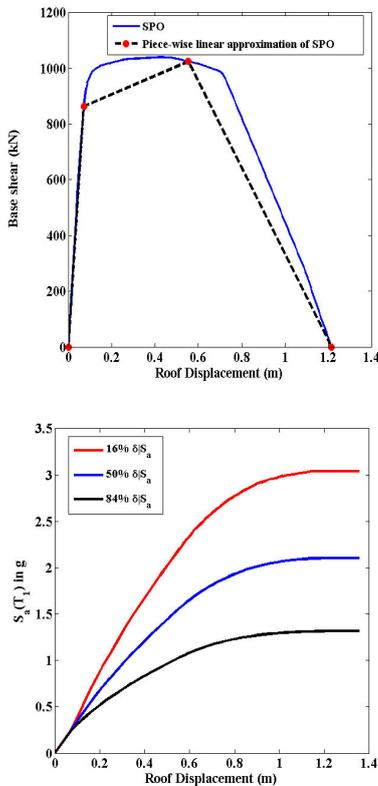
Figure 4: Pushover curves, piece-wise linear approximations and approximate IDA from SPO2IDA (adopted from Rajeev et al., 2014)
