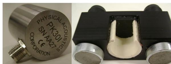
(a) An acoustic emission sensor (b) A spring-loaded magnetic holder
