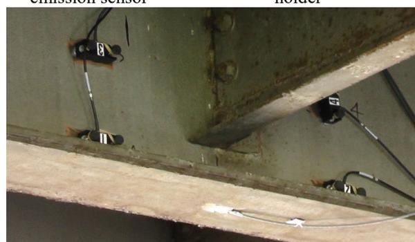
(c) AE sensors mounted on a steel girder
