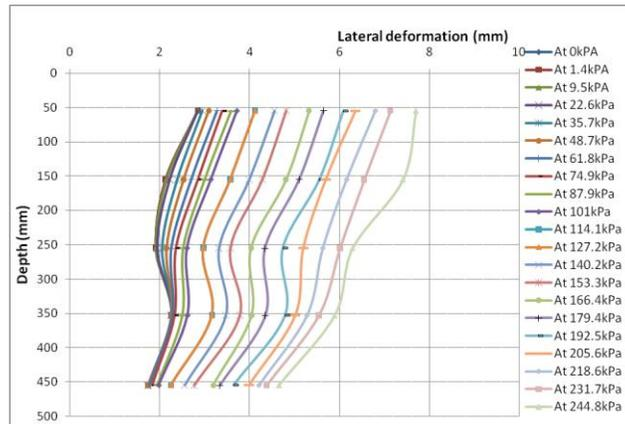
Figure 9. Vertical profile of geotextile reinforced wall during the reloading stage at natural moisture content
