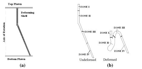
Fig. 3(a). Computational model for axisymmetric deformation, (b) Demarcation of zones in undeformed and a typically deformed shell
