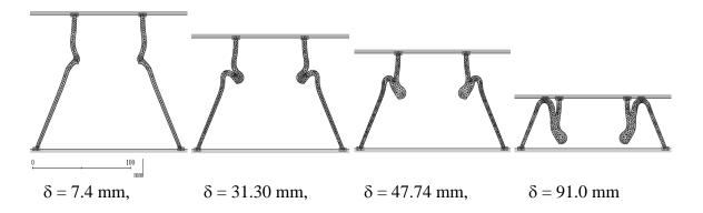
Fig. 4 Typical computed deformed profiles at different values of compression ( $\delta$ ).
