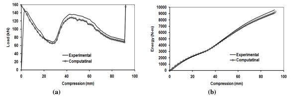
Fig. 2 Comparison of typical (a) load-compression and (b) energy-compression curves for shells.
