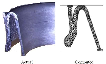
Fig. 5 Comparison of deformed shapes of specimen F5 after compression.
