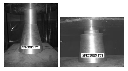
Fig. 1 Typical views of the undeformed and deformed shells.
