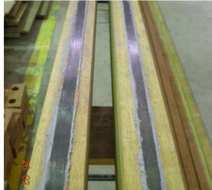
**Figure 4** Strengthened timber beams being cured in the lab
