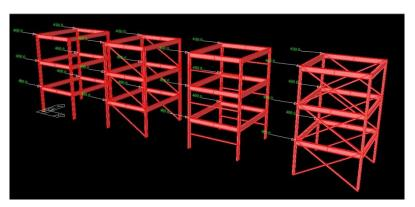
reconstruct the structures especially bracing systems in order to strengthen it after considering the environment of the building that is to be built. Thus, with this program, four different buildings were also set up with various bracings. Then, for each of the bar, the force of 400N was applied in order to give a horizontal force similar to the spaghetti noddle experiment.
