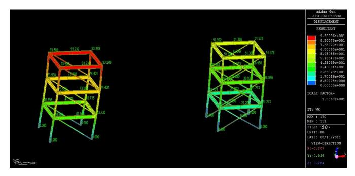
This picture clearly shows the different between X and Diagonal bracings.
