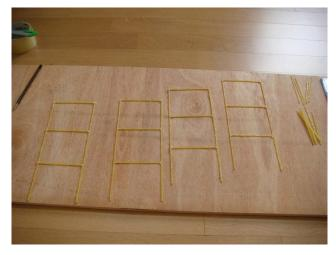
noodles by using the glue, vary the types of bracing: none, X, diagonal, and a parallel line. Measure the length of the horizontal and vertical spaghetti noodles.
