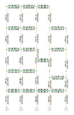
Fig.6. Required Column reinforcement mm<sup>2</sup> for a frame in XZ plane at
