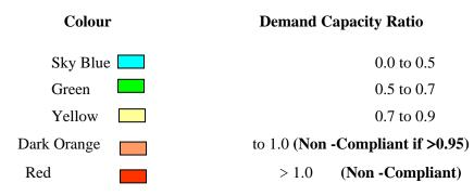
The demand capacity ratios are particularly of significance to the columns and they are also indicated as Column P-M-M Interaction Ratios by SAP.
