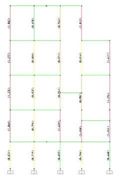
Fig.5. Column Demand Capacity Ratios in for a frame in XZ plane at Y=0m Y=0m
