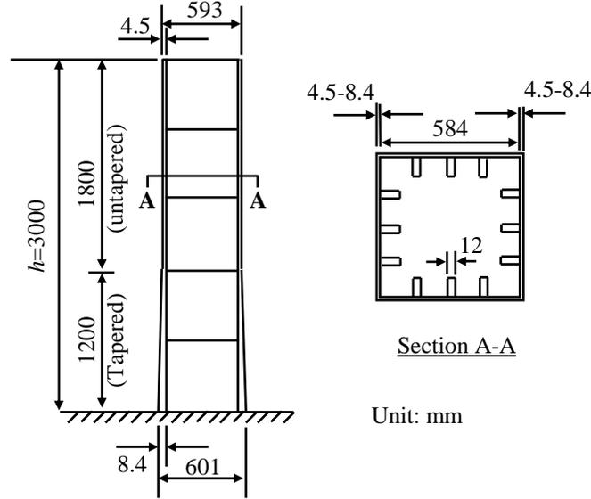
Figure 1. Dimensions of tapered plate steel column
