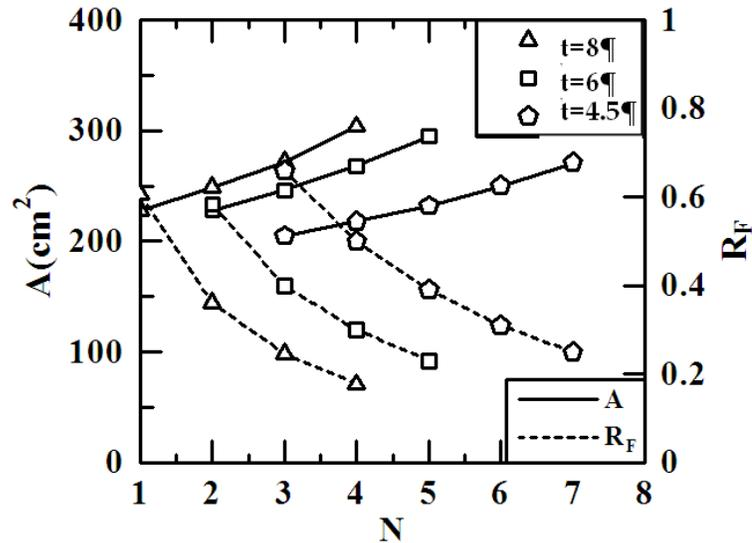
Figure 3. Variations of  $A$  and  $R_F$  with number of ribs,  $N$
