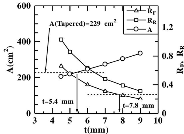
Figure 2 Variations of  $A$ ,  $R_F$ ,  $R_R$  with thickness of plates
