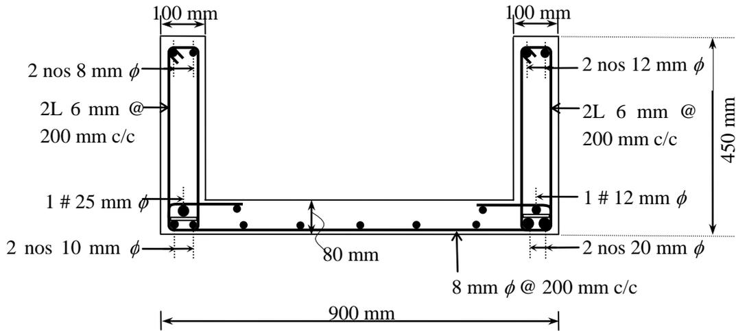
Figure 2: Reinforcement details of test beams with slab connection on flexural tension side
