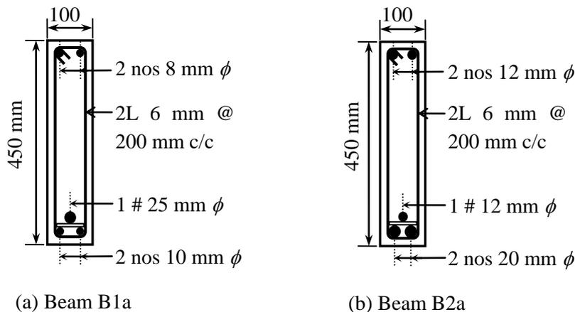
Figure 1: Reinforcement details of rectangular test beams
