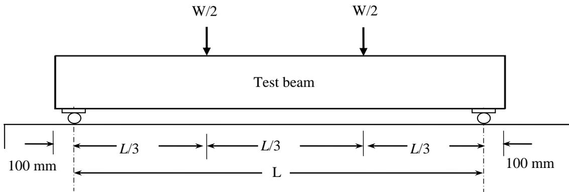
Figure 4: Load position for test beams
