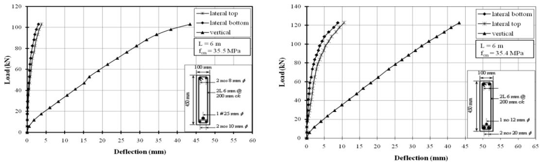
Figure 4: Mid-span deflection for beams B1a and B2a
