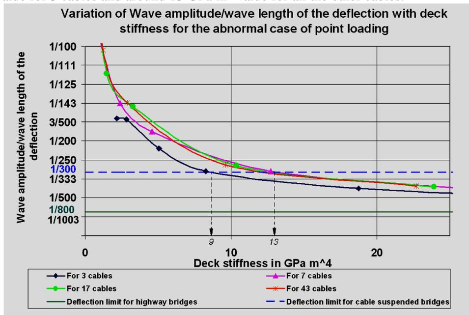
Fig 3.4 Variation of (wave amplitude/wave length) of the deflection with deck stiffness for the abnormal type of load case
