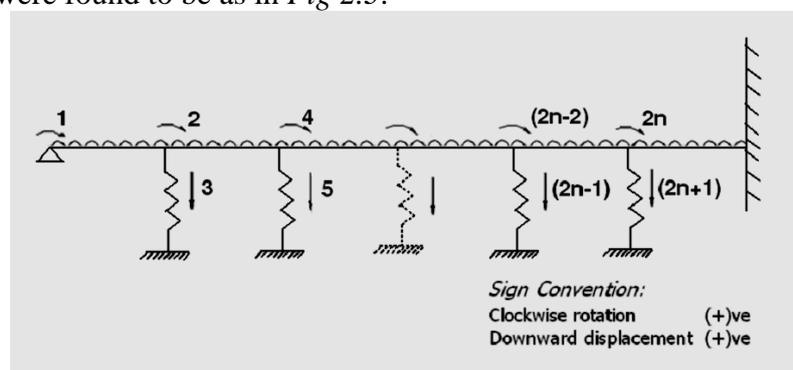
Fig 2.3 Joint rotations and displacement along the bridge deck
