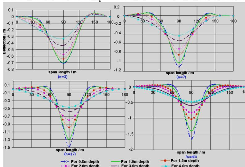
Fig 3.3 Variation of deflection with span length for different number of cables for the abnormal type of loading
