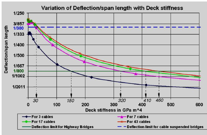
Fig 3.2 Variation of (deflection/span length) with deck stiffness for different number of cables for the uniformly distributed type of load throughout the bridge deck
