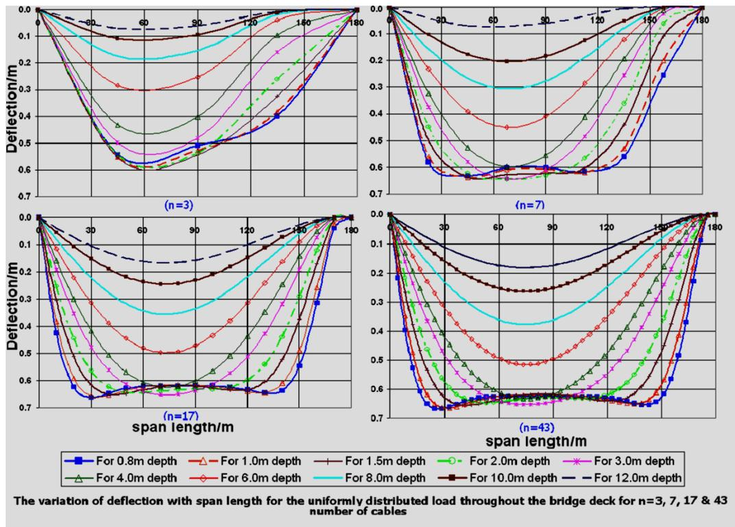
Fig 3.1 Comparison of the variation of deflection with span length for different number of cables for the uniformly distributed load throughout the bridge
