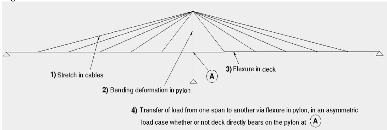
*Fig 2.1 The deck stiffness guidance factors*
