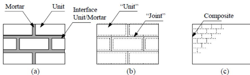
**Figure 2: Modelling strategies for masonry structures: (a) detailed micro-modelling; (b) simplified micro-modelling; (c) macro-modelling (Lourenco, 1999)**
