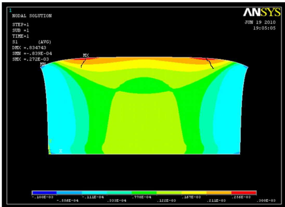
*Figure 5: Principal stress contour diagrams generated through the mathematical models developed for M1 and M2*
