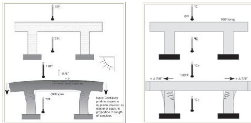
**Figure 1: Cracking of masonry wall due to thermal movements of an overlying slab (Dilrukshi & Dias 2008)**
