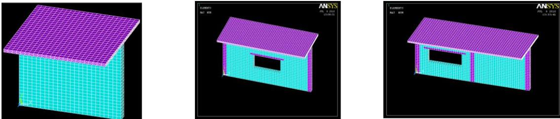
*Figure 4: Few idealised assemblies used in the finite element model*
