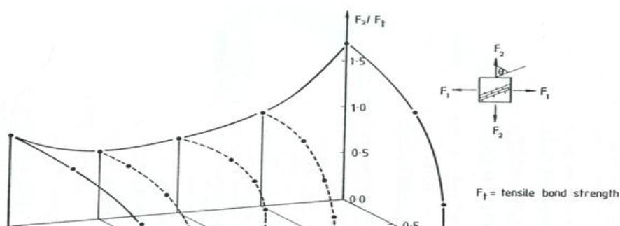
*Figure 3: Biaxial stress failure envelope developed by Page (1980)*
