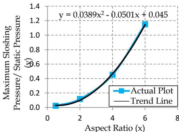
Fig 10: Variation of normalized sloshing pressure with aspect ratio
