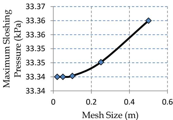
Fig 7: Variation of sloshing pressure with mesh size
