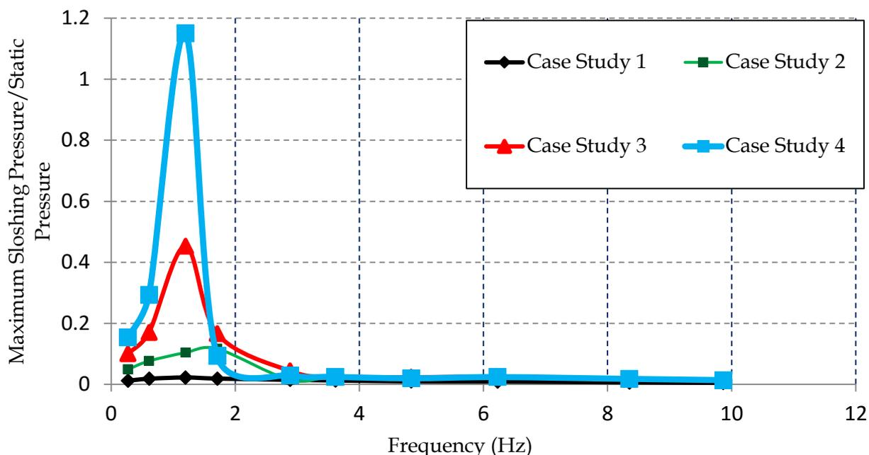
Fig 9: Variation of normalized sloshing pressure with frequency
