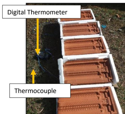
Figure 2 : Testing thermal properties
