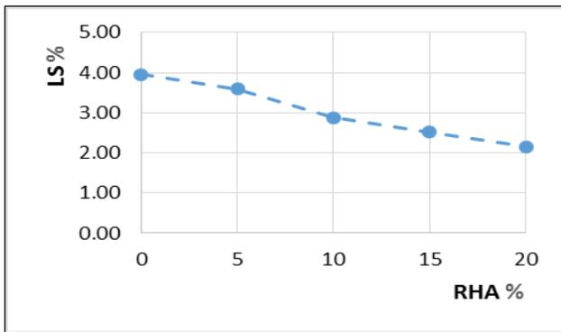
Figure 7 : Variation in Linear Shrinkage with RHA %
