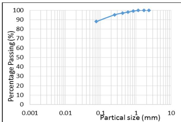
Figure 4 : Particle size Distribution of Clay
