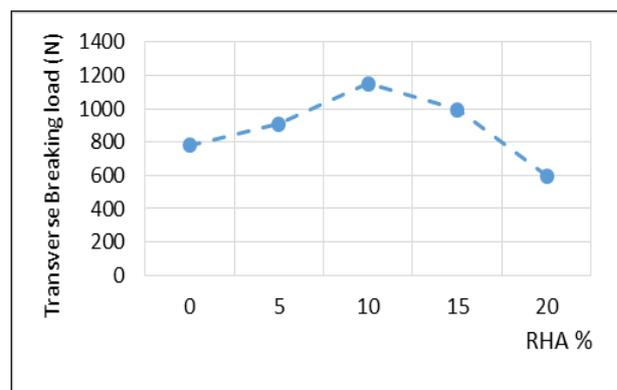
Figure 8 : Variation in Transverse Breaking Load with RHA %
