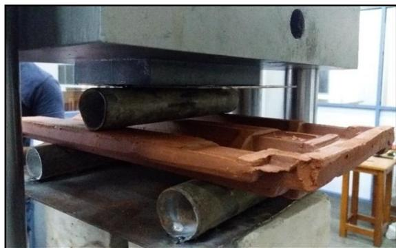
Figure 1 : Arrangement of specimen for transverse test
