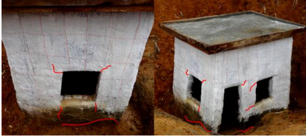
Fig 9: Observed crack lines after blasting
