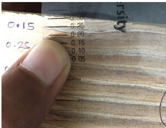
Figure 9: Observing the crack width using gauge
