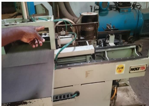
Figure 2: Sample preparation using finger cutting machine
