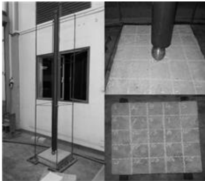
Fig 03: Instrumental setup for the impact resistance test
