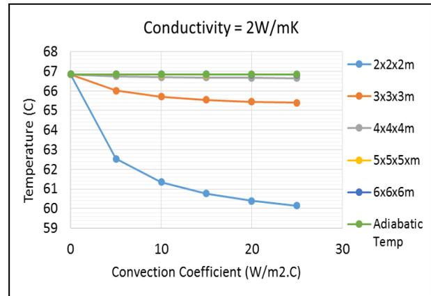
Figure 7: Temperature at the core for Conductivity of 2W/mk
