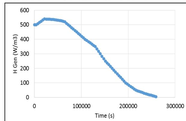
Figure 5: Rate of heat generation with time used to simulate temperature rise
