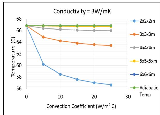
Figure 8: Temperature at the core for Conductivity of 3W/mK.
