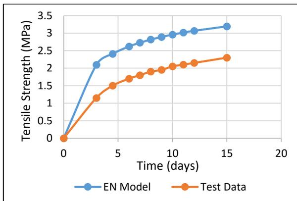
Figure 3: Tensile Strength variation with Time
