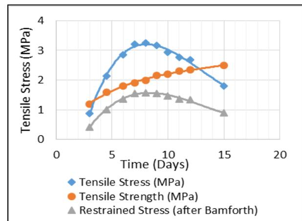
Figure 6: Tensile Stress obtained by FE analysis, Tensile Strength and Restrained Stress variation with Time
