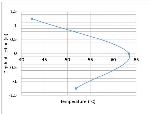
Figure 1: Temperature distribution across the depth of a 3m thick block at 7 days
