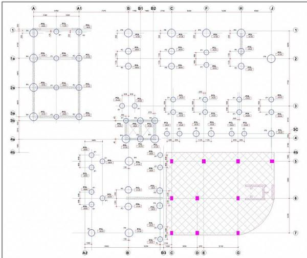
Figure 1: Pile layout
