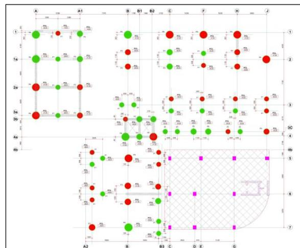
Figure 2: Layout of piles based on soft toe condition
