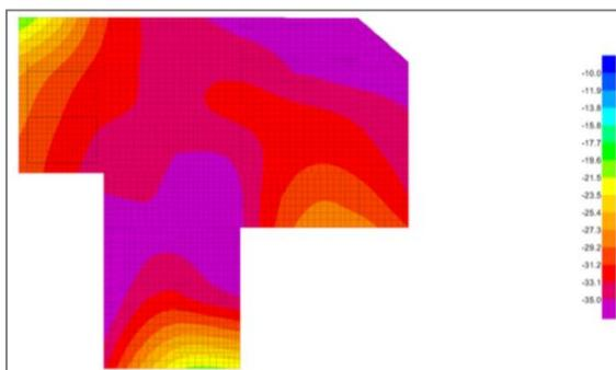
Figure 4: Deformation diagram of raft (in millimetres)
