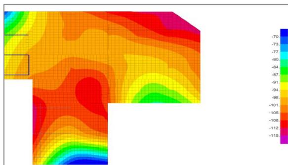
Figure 5: Soil pressure diagram of raft (in kN/m<sup>2</sup>)
