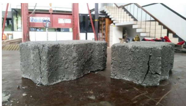
Fig. 05. Failure mode of sample paving blocks
