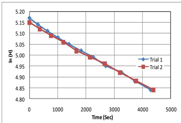
Fig. 6: Results of permeability test (Falling head)
