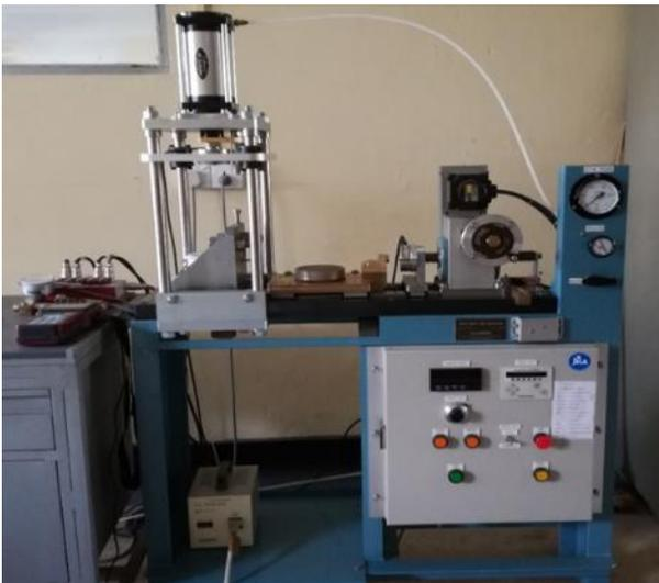
Fig. 3. Automated Direct Shear Apparatus
