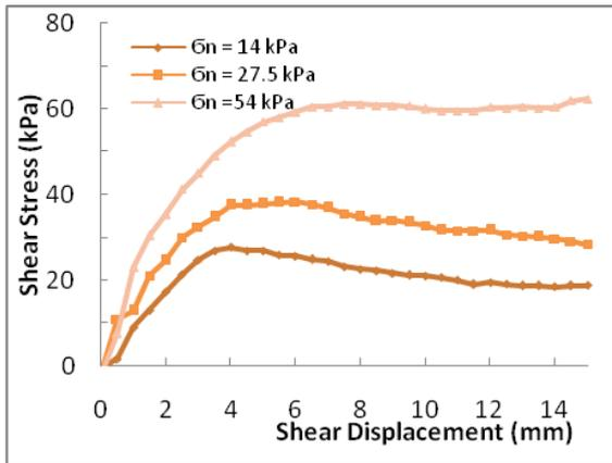
Fig. 7: Variation of shear stress with shear displacement
