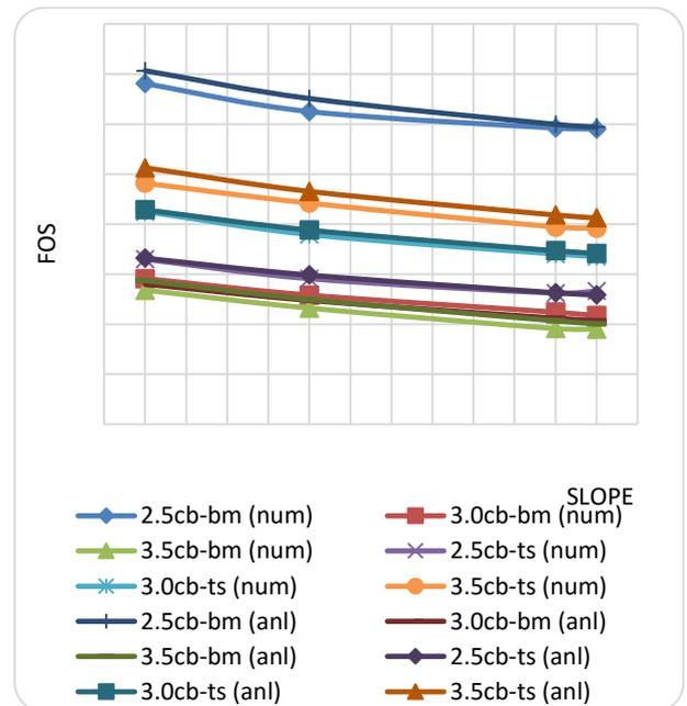
Fig. 15: Variation of FOS with slope angle obtained numerically for circular failure modes
