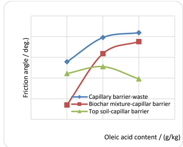
Fig. 10: Variation of friction angle with oleic acid content of capillary barrier (cb)
