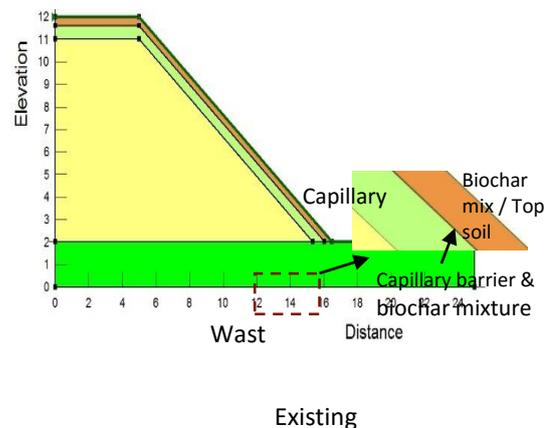
Fig.11. Configuration of the landfill used in Slope/W
