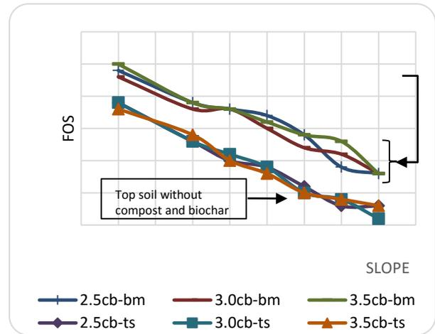
Fig. 14: Variation of FOS with slope angle obtained numerically and analytically for block and infinite failure modes respectively
