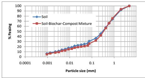
Fig. 5: Particle size distribution of top soil and biochar-compost mixed top soil
