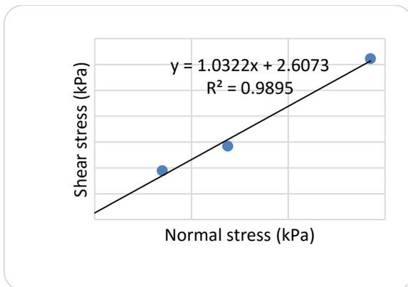
Fig. 8: Variation of peak shear stress with normal stress
