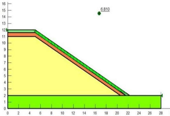
Fig. 13: Critical Block failure surface analysis
