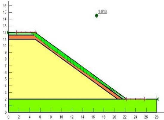
Fig. 12. Critical failure surface corresponding to circular slip surface
