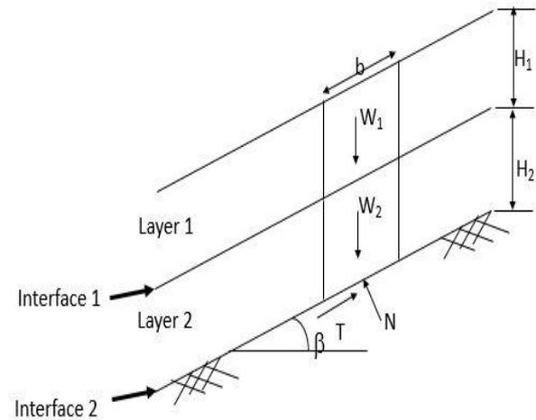
Fig. 4: configuration of the capping layer consisting of two materials and relevant interfaces
