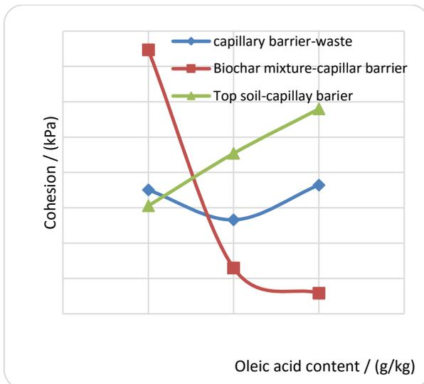
Fig. 9: Variation of cohesion with oleic acid content of capillary barrier
