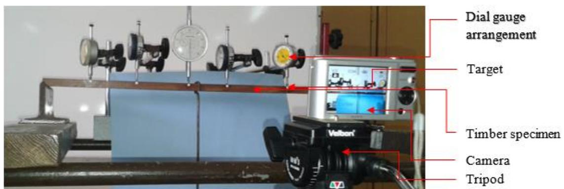
Figure 8: Experimental setup of bending test
