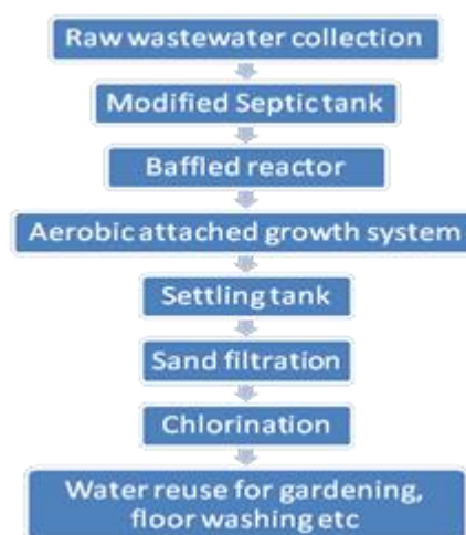
Fig. 2 Sequential flow diagram of onsite wastewater treatment system
