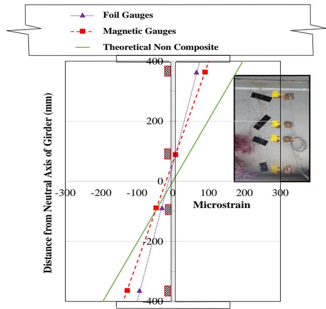
Fig. 09: Magnetic strain gauge results
