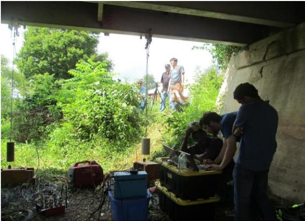
Fig. 10: Sensor equipment underneath the bridge
