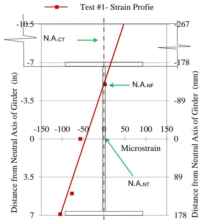
Fig. 05: Strain readings at mid-span
