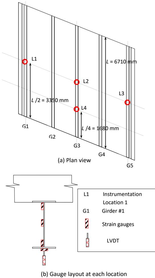
Fig. 03: Strain gauge and LVDT layout
