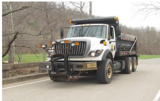
Fig. 08: Loaded dump truck placed on deck
