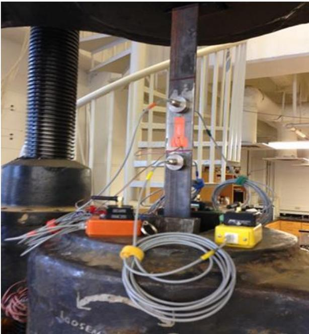
Fig. 06: Magnetic strain gauge calibration
