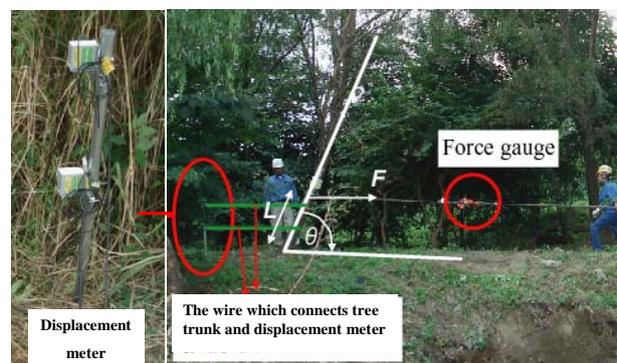
Fig.2 Layout of tree-pulling system
