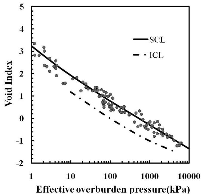
Figure 2: Normalized compression curves for several clays (from Skempton [3]) in showing the intrinsic compression line (ICL) and sedimentation compression line (SCL) (from Burland [1])
