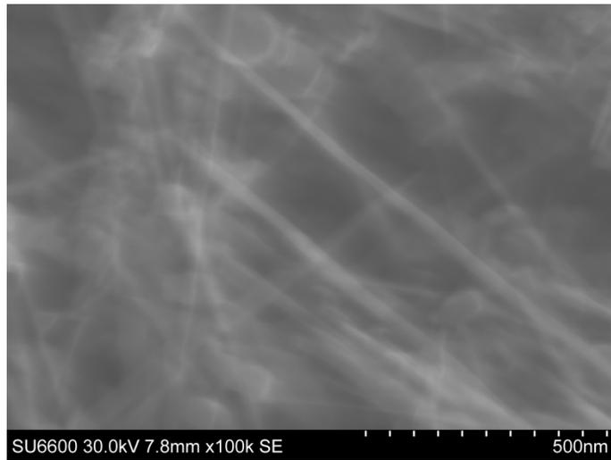
**Fig. 4:** SEM image of the produced CNTs
