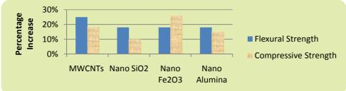
**Fig. 5**: Percentage increase in Compressive and Flexural Strengths with the addition of nano Particles (Sobolev et al., 2009, Hosseini et al., 2009, Vera-Agullo et al., 2009, Sanchez and Sobolev, 2010), Metaxa et al, Nazari et al., 2010b, Nazari et al., 2010c)
