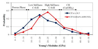
**Fig.2**: Probability plot of Young's Modulus of 28 days cement paste(w/c=0.5) and cement paste reinforced with 0.08wt% MWCNTs (Metaxa et al.)
