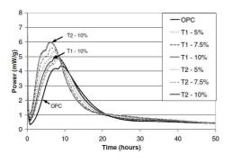
Fig. 4: Rate of Hydration of TiO<sub>2</sub> –blended cements (Jayapalan et al., 2009)
