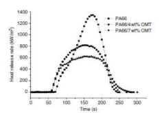
Fig. 10: Comparison of heat Release rates, PA66 and PA66/OMT nanocomposites (Song et al., 2008).
