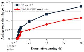
**Fig.3**: Autogenous shrinkage of cement paste (w/c=0.3) and cement paste reinforced with 0.048wt% MWCNTs (Metaxa et al.)
