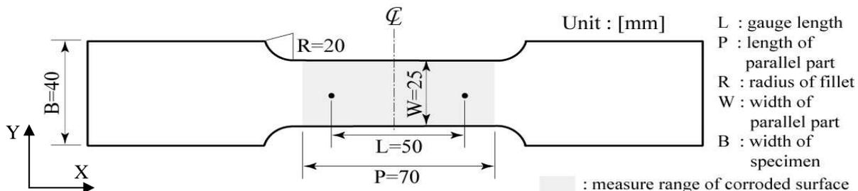
Figure 1: JIS No.5 Specimen for tensile test
