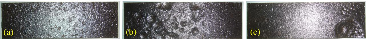
Figure 4: Plates with (a) minor corrosion (F-14), (b) moderate corrosion (F-13) and (c) severe corrosion (F-19)
