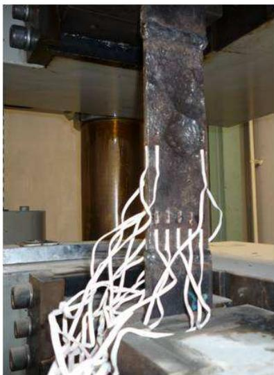
Figure 2: Specimen prepared for the tensile test
