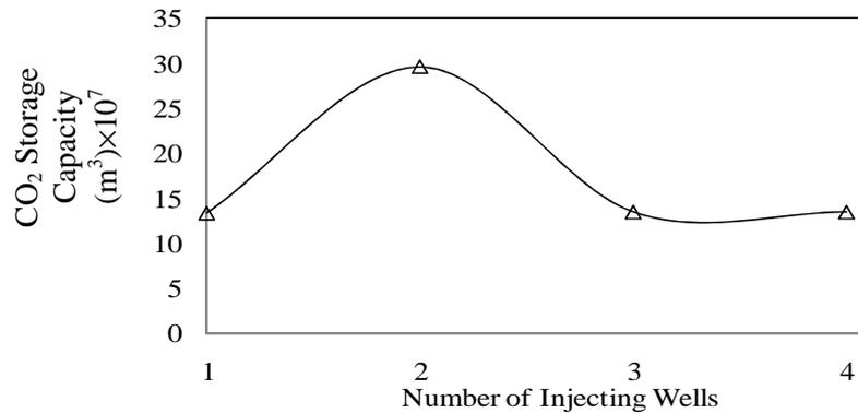
Figure 4. Variation CO<sub>2</sub> storage capacity with number of injecting wells.
