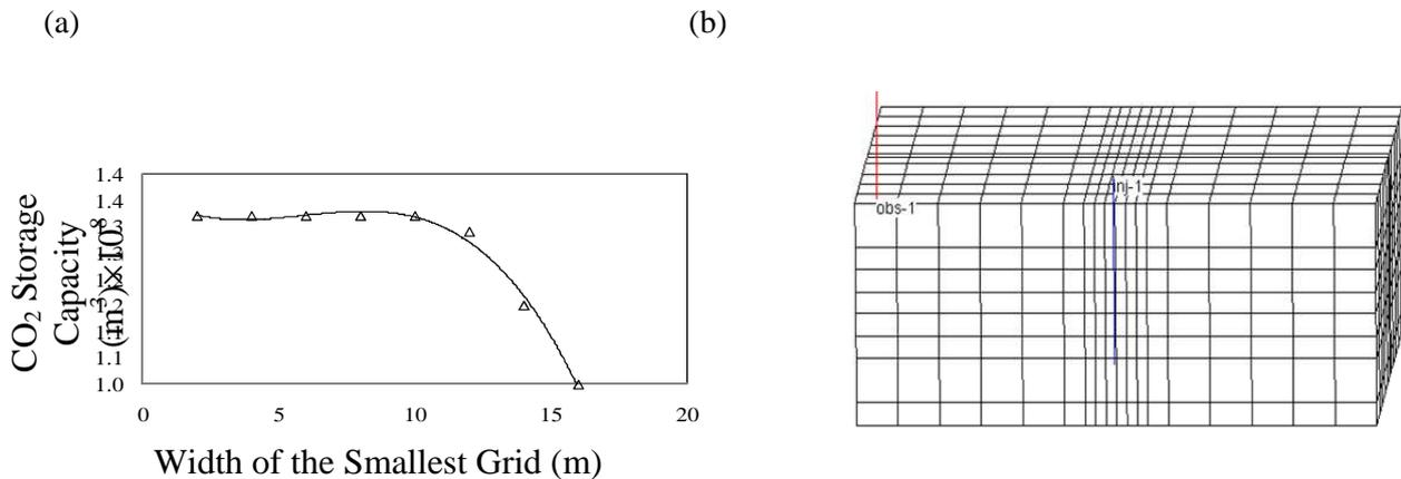
Figure 2. (a) Effects of grid size on storage, and (b) selected model grid blocks for the coal seam.
