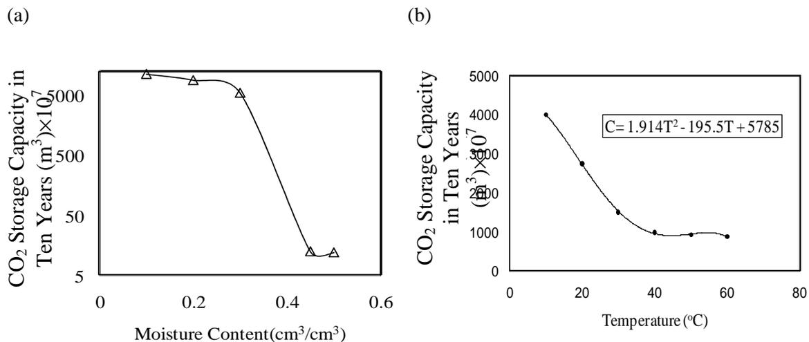
Figure 6. Variation of CO<sub>2</sub> storage capacity of coal mass for 10 years of injection with the (a) coal bed moisture content and (b) coal bed temperature.
