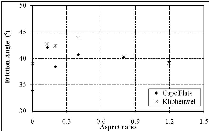
**Figure 4.** *The friction angle versus aspect ratio (after Petersen, 2009)*
