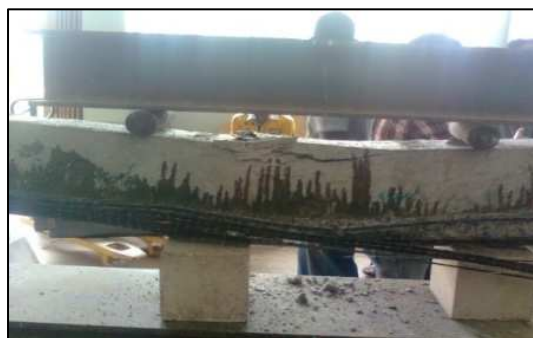
Figure 6: Concrete crushing and de-bonding of FRP bonded beam
