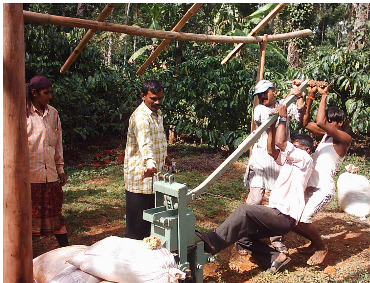
Fig. 2 – Production of compacted SMB using manual press
