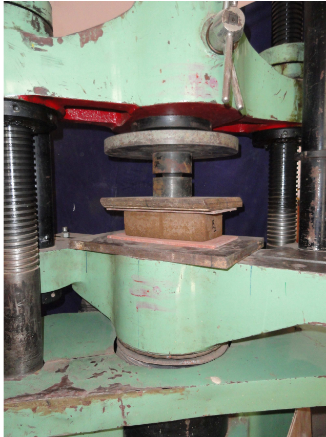
Fig. 3 – Brick under wet compressive strength test
