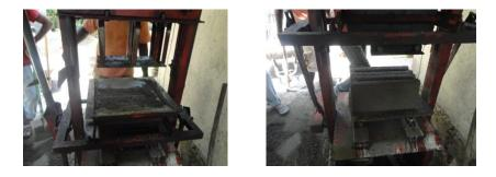
Figure 2: Block Manufacturing
