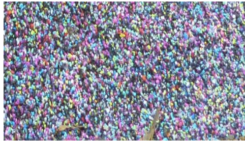
Figure 1: Rubber sample used to fill the trench
