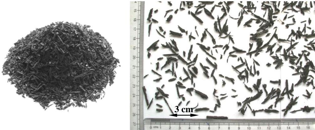
*Figure 1: Rubber fibres used (retained between 4.75 and 2 mm size sieves)*
