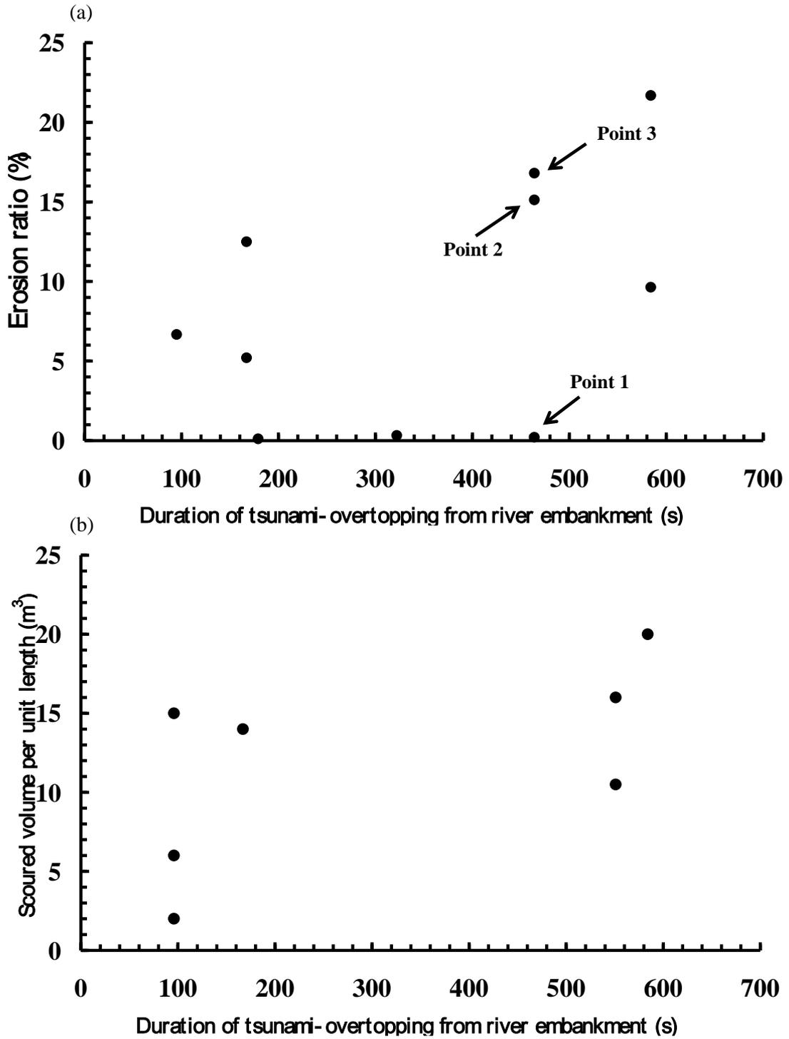
Figure 7: Relationship between overtopping time and (a) erosion ratio and (b) scoured volume. (Locations of Point 1, 2 and 3 are shown in Figure 8. Definition of the parameter in vertical axis is shown in Figure 2.)
