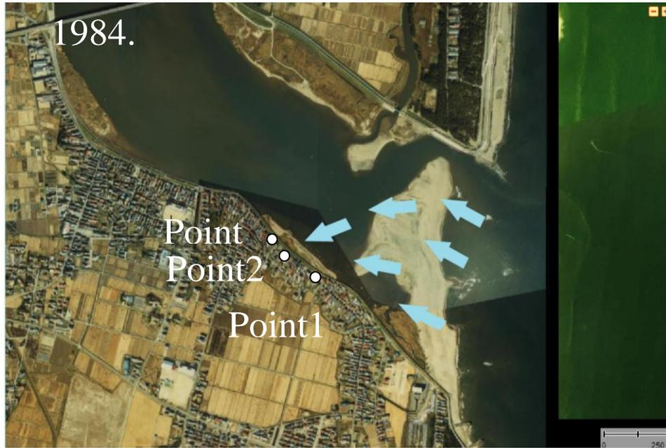
Figure 8: The change of Tsunami direction due to the sand bar. Point 1, 2 and 3 are shown the location related to the plots in Figure 7(a). Although a sand bar shown in the aerial photo before tsunami is old, the sand bar existed just before the tsunami came. (Modified the aerial photo provided by Geospatial Information Authority of Japan)
