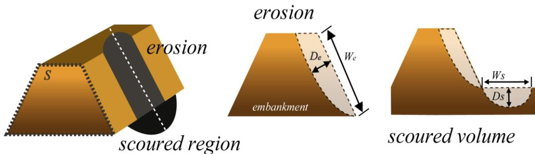
Figure 2: Definition of observed parameters regarding erosion and scouring.
